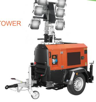
Our Eco8 units come with 6 multi-directional 160W, 48V LED lights offering an illumination area of 4,200sqm and a running time of up to 200 hours. – maximising safety, good value, uptime and efficiency while minimising costs, pollutants and CO2 emissions.
